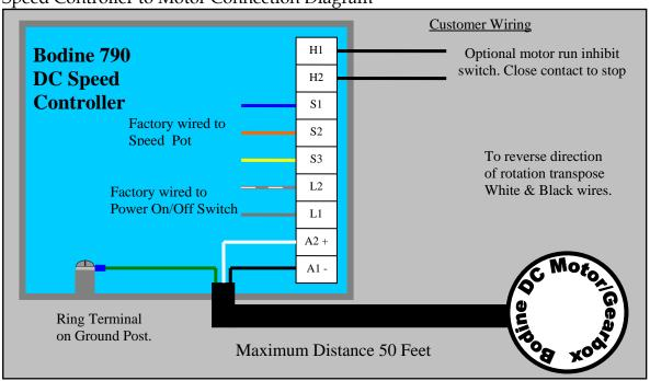
Motor Wiring to Bodine 790 Speed Controller
